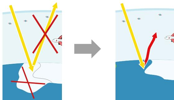
Explanation: If the ice surface disappears, the ray of light impinges onto the water surface and will not be reflected, but transformed into a ray of heat.
